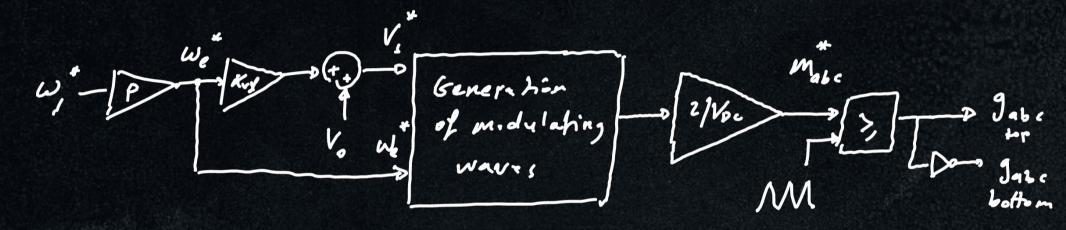
$m_{a}^{*} = \sqrt{2} V_{s} \sin(\omega_{e}^{*}t) \frac{2}{V_{DC}}$   $m_{b}^{*} = \sqrt{2} V_{s} \sin(\omega_{e}^{*}t - 2\pi/2) \frac{2}{V_{DC}}$   $m_{c}^{*} = \sqrt{2} V_{s} \sin(\omega_{e}^{*}t + 2\pi/3) \frac{2}{V_{DC}}$
