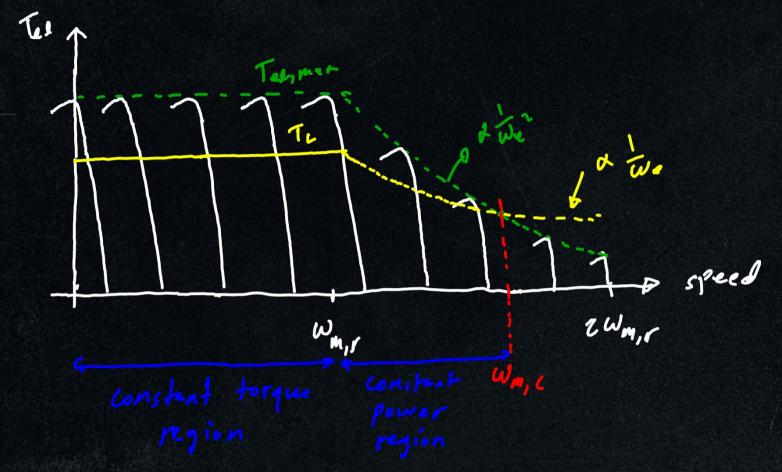
In the constant power mode, the torque keeps decreasing inversely with speed. At critical speed, wmc, the maximum tarque is reached. Any aftempt to operate beyond this speed will stall the motor. This is the limit of constant power region.
