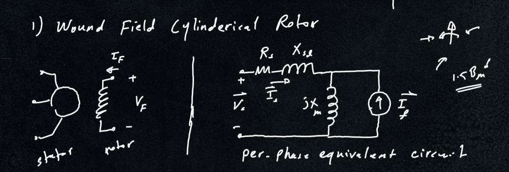
. The peak of rotating mmf produced by the rm current, If flowing through  $N_a$  turns is  $F_1 = \frac{3}{2} N_a (\sqrt{2} I_z)$ . The peak of rotating mmf produced by a dc current  $I_F$  flowing through  $N_f$  turns is  $F_2 = N_f I_F$   $F_1 = F_1 \quad \text{D} \quad I_g = N I_F \quad \text{where} \quad N = \frac{\sqrt{2}}{3} \frac{N_f}{N_a}$
